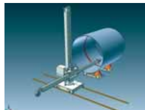
Inner peripheral welding (with the rotator)
