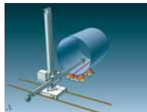
Inner linear welding (by the movement of the boom)
