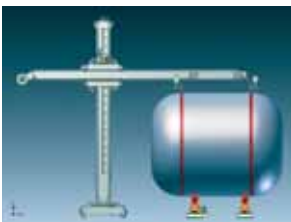
Outer peripheral welding by using the double welding head (with the rotator)
