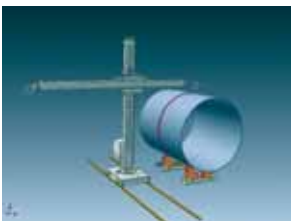
Outer peripheral welding (with the rotator)
